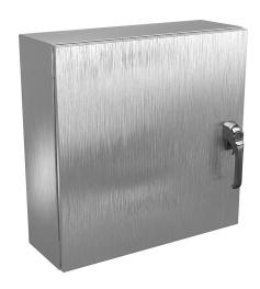
Wiegmann Ultimate series enclosure, NEMA 4X/12/13,  $24 \times 24 \times 8$  in (HxWxD), wall mount, 304 stainless steel, No. 3 intermediate polished finish, single-door, 3-point 316L padlocking handle.
