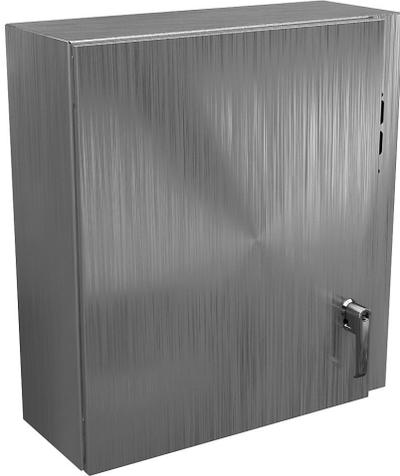
Wiegmann Ultimate series disconnect enclosure, NEMA 4/4X/12/13, right flange, 24 x 22 x 8in (HxWxD), wall mount, 304 stainless steel, No. 3 intermediate polished finish, single-door, 2-point padlocking handle, purchase subpanel separately.
