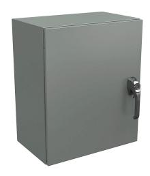
Wiegmann Ultimate series enclosure, NEMA 4/12/13, 24 x 20 x 12in (HxWxD), wall mount, carbon steel, ANSI 61 gray, powder coat finish, single-door, 3-point keylocking/padlocking combo handle.
