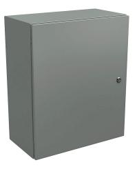
Wiegmann Ultimate series enclosure, NEMA 4/12/13, 24 x 20 x 10in (HxWxD), wall mount, carbon steel, ANSI 61 gray, powder coat finish, single-door, 1/4-turn semi-flush oil-tight latch.
