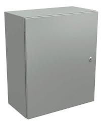
Wiegmann Ultimate series enclosure, NEMA 4/12/13, 24 x 20 x 10in (HxWxD), wall mount, carbon steel, RAL 7035 light gray, powder coat finish, single-door, 1/4-turn semi-flush oil-tight latch.
