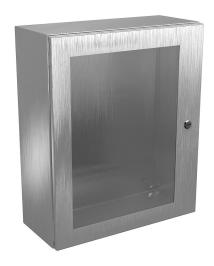
Wiegmann Ultimate series enclosure, NEMA 4/4X/12/13,  $24 \times 20 \times 8$  in (HxWxD), wall mount, 304 stainless steel, No. 3 intermediate polished finish, single-door, 1/4-turn semi-flush oil-tight latch, polycarbonate window.
