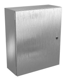
Wiegmann Ultimate series enclosure, NEMA 4/4X/12/13,  $24 \times 20 \times 8$  in (HxWxD), wall mount, 316L stainless steel, No. 3 intermediate polished finish, single-door, 1/4-turn semi-flush oil-tight latch.
