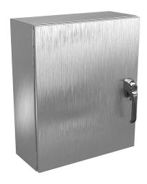
Wiegmann Ultimate series enclosure, NEMA 4X/12/13, 24 x 20 x 8in (HxWxD), wall mount, 304 stainless steel, No. 3 intermediate polished finish, single-door, 3-point 316L padlocking handle.
