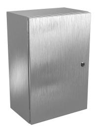
Wiegmann Ultimate series enclosure, NEMA 4/4X/12/13,  $24 \times 16 \times 10$  in (HxWxD), wall mount, 304 stainless steel, No. 3 intermediate polished finish, single-door, 1/4-turn semi-flush oil-tight latch.
