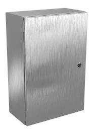
Wiegmann Ultimate series enclosure, NEMA 4/4X/12/13,  $24 \times 16 \times 8$ in (HxWxD), wall mount, 304 stainless steel, No. 3 intermediate polished finish, single-door, 1/4-turn semi-flush oil-tight latch.
