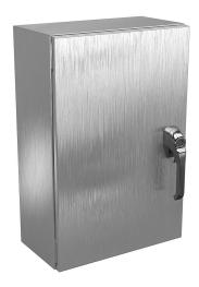
Wiegmann Ultimate series enclosure, NEMA 4X/12/13, 24 x 16 x 8in (HxWxD), wall mount, 304 stainless steel, No. 3 intermediate polished finish, single-door, 3-point 316L padlocking handle.
