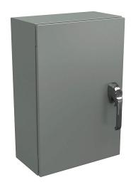
Wiegmann Ultimate series enclosure, NEMA 4/12/13, 24 x 16 x 8in (HxWxD), wall mount, carbon steel, ANSI 61 gray, powder coat finish, single-door, 3-point keylocking/padlocking combo handle.
