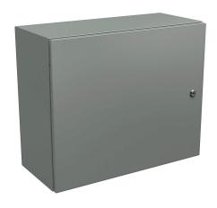
Wiegmann Ultimate series enclosure, NEMA 4/12/13, 20 x 24 x 10in (HxWxD), wall mount, carbon steel, ANSI 61 gray, powder coat finish, single-door, 1/4-turn semi-flush oil-tight latch.
