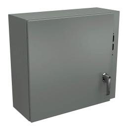
Wiegmann Ultimate series disconnect enclosure, NEMA 4/12/13, right flange, 20 x 22 x 8in (HxWxD), wall mount, carbon steel, ANSI 61 gray, powder coat finish, single-door, 2-point padlocking handle, purchase subpanel separately.
