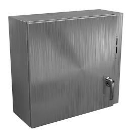
Wiegmann Ultimate series disconnect enclosure, NEMA 4/4X/12/13, right flange, 20 x 22 x 8in (HxWxD), wall mount, 316L stainless steel, No. 3 intermediate polished finish, single-door, 2-point padlocking handle, purchase subpanel separately.
