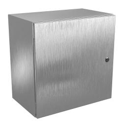
Wiegmann Ultimate series enclosure, NEMA 4/4X/12/13, 20 x 20 x 12in (HxWxD), wall mount, 304 stainless steel, No. 3 intermediate polished finish, single-door, 1/4-turn semi-flush oil-tight latch.
