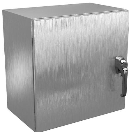
Wiegmann Ultimate series enclosure, NEMA 4X/12/13, 20 x 20 x 12in (HxWxD), wall mount, 304 stainless steel, No. 3 intermediate polished finish, single-door, 1-point 316L padlocking handle.
