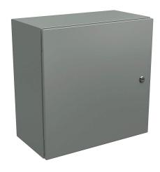
Wiegmann Ultimate series enclosure, NEMA 4/12/13, 20 x 20 x 10in (HxWxD), wall mount, carbon steel, ANSI 61 gray, powder coat finish, single-door, 1/4-turn semi-flush oil-tight latch.
