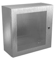
Wiegmann Ultimate series enclosure, NEMA 4/4X/12/13, 20 x 20 x 8in (HxWxD), wall mount, 304 stainless steel, No. 3 intermediate polished finish, single-door, 1/4-turn semi-flush oil-tight latch, polycarbonate window.
