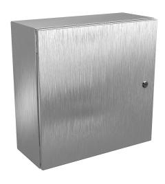
Wiegmann Ultimate series enclosure, NEMA 4/4X/12/13,  $20 \times 20 \times 8$ in (HxWxD), wall mount, 304 stainless steel, No. 3 intermediate polished finish, single-door, 1/4-turn semi-flush oil-tight latch.
