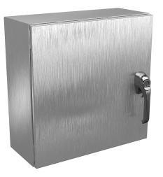
Wiegmann Ultimate series enclosure, NEMA 4X/12/13, 20 x 20 x 8in (HxWxD), wall mount, 304 stainless steel, No. 3 intermediate polished finish, single-door, 1-point 316L padlocking handle.
