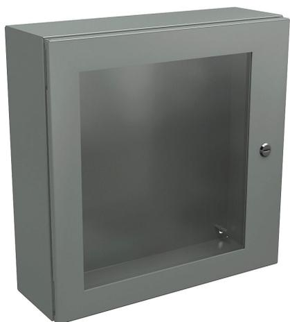
Wiegmann Ultimate series enclosure, NEMA 4/12/13, 20 x 20 x 6in (HxWxD), wall mount, carbon steel, ANSI 61 gray, powder coat finish, single-door, 1/4-turn semi-flush oil-tight latch, polycarbonate window.
