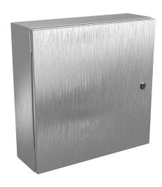
Wiegmann Ultimate series enclosure, NEMA 4/4X/12/13, 20 x 20 x 6in (HxWxD), wall mount, 304 stainless steel, No. 3 intermediate polished finish, single-door, 1/4-turn semi-flush oil-tight latch.
