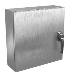
Wiegmann Ultimate series enclosure, NEMA 4X/12/13,  $20 \times 20 \times 6$  in (HxWxD), wall mount, 304 stainless steel, No. 3 intermediate polished finish, single-door, 1-point 316L padlocking handle.
