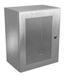
Wiegmann Ultimate series enclosure, NEMA 4/4X/12/13,  $20 \times 16 \times 10$  in (HxWxD), wall mount, 304 stainless steel, No. 3 intermediate polished finish, single-door, 1/4-turn semi-flush oil-tight latch, polycarbonate window.
