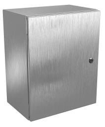
Wiegmann Ultimate series enclosure, NEMA 4/4X/12/13, 20 x 16 x 10in (HxWxD), wall mount, 304 stainless steel, No. 3 intermediate polished finish, single-door, 1/4-turn semi-flush oil-tight latch.
