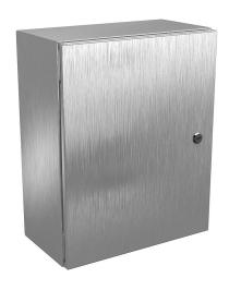
Wiegmann Ultimate series enclosure, NEMA 4/4X/12/13, 20 x 16 x 8in (HxWxD), wall mount, 304 stainless steel, No. 3 intermediate polished finish, single-door, 1/4-turn semi-flush oil-tight latch.
