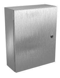
Wiegmann Ultimate series enclosure, NEMA 4/4X/12/13, 20 x 16 x 6in (HxWxD), wall mount, 304 stainless steel, No. 3 intermediate polished finish, single-door, 1/4-turn semi-flush oil-tight latch.
