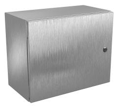
Wiegmann Ultimate series enclosure, NEMA 4/4X/12/13, 16 x 20 x 10in (HxWxD), wall mount, 304 stainless steel, No. 3 intermediate polished finish, single-door, 1/4-turn semi-flush oil-tight latch.
