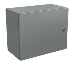
Wiegmann Ultimate series enclosure, NEMA 4/12/13, 16 x 20 x 10in (HxWxD), wall mount, carbon steel, ANSI 61 gray, powder coat finish, single-door, 1/4-turn semi-flush oil-tight latch.
