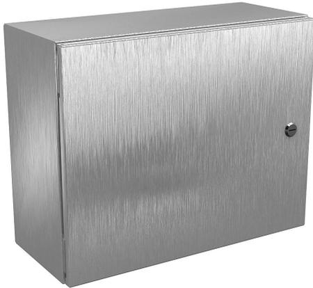
Wiegmann Ultimate series enclosure, NEMA 4/4X/12/13, 16 x 20 x 8in (HxWxD), wall mount, 304 stainless steel, No. 3 intermediate polished finish, single-door, 1/4-turn semi-flush oil-tight latch.
