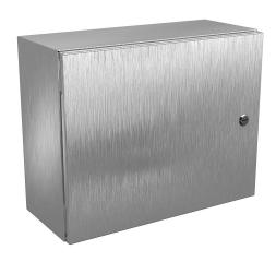
Wiegmann Ultimate series enclosure, NEMA 4/4X/12/13,  $16 \times 20 \times 8$  in (HxWxD), wall mount, 316L stainless steel, No. 3 intermediate polished finish, single-door, 1/4-turn semi-flush oil-tight latch.
