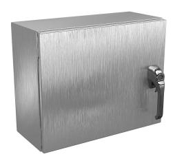
Wiegmann Ultimate series enclosure, NEMA 4X/12/13, 16 x 20 x 8in (HxWxD), wall mount, 316L stainless steel, No. 3 intermediate polished finish, single-door, 1-point 316L padlocking handle.
