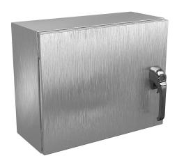
Wiegmann Ultimate series enclosure, NEMA 4X/12/13,  $16 \times 20 \times 8$  in (HxWxD), wall mount, 304 stainless steel, No. 3 intermediate polished finish, single-door, 1-point 316L padlocking handle.
