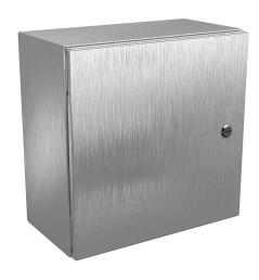
Wiegmann Ultimate series enclosure, NEMA 4/4X/12/13, 16 x 16 x 8in (HxWxD), wall mount, 304 stainless steel, No. 3 intermediate polished finish, single-door, 1/4-turn semi-flush oil-tight latch.
