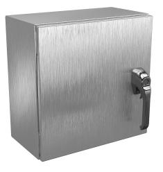
Wiegmann Ultimate series enclosure, NEMA 4X/12/13, 16 x 16 x 8in (HxWxD), wall mount, 304 stainless steel, No. 3 intermediate polished finish, single-door, 1-point 316L padlocking handle.
