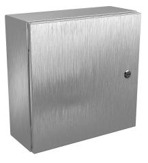
Wiegmann Ultimate series enclosure, NEMA 4/4X/12/13, 16 x 16 x 6in (HxWxD), wall mount, 304 stainless steel, No. 3 intermediate polished finish, single-door, 1/4-turn semi-flush oil-tight latch.
