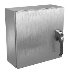
Wiegmann Ultimate series enclosure, NEMA 4X/12/13, 16 x 16 x 6in (HxWxD), wall mount, 316L stainless steel, No. 3 intermediate polished finish, single-door, 1-point 316L padlocking handle.
