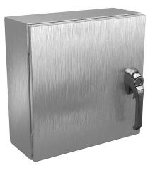
Wiegmann Ultimate series enclosure, NEMA 4X/12/13,  $16 \times 16 \times 6$  in (HxWxD), wall mount, 316L stainless steel, No. 3 intermediate polished finish, single-door, 1-point 316L padlocking handle.
