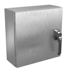
Wiegmann Ultimate series enclosure, NEMA 4X/12/13,  $16 \times 16 \times 16$  (HxWxD), wall mount, 304 stainless steel, No. 3 intermediate polished finish, single-door, 1-point 316L padlocking handle.
