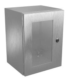
Wiegmann Ultimate series enclosure, NEMA 4/4X/12/13,  $16 \times 12 \times 10$  in (HxWxD), wall mount, 304 stainless steel, No. 3 intermediate polished finish, single-door, 1/4-turn semi-flush oil-tight latch, polycarbonate window.
