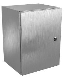
Wiegmann Ultimate series enclosure, NEMA 4/4X/12/13, 16 x 12 x 10in (HxWxD), wall mount, 304 stainless steel, No. 3 intermediate polished finish, single-door, 1/4-turn semi-flush oil-tight latch.
