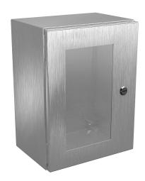
Wiegmann Ultimate series enclosure, NEMA 4/4X/12/13,  $16 \times 12 \times 8$  in (HxWxD), wall mount, 304 stainless steel, No. 3 intermediate polished finish, single-door, 1/4-turn semi-flush oil-tight latch, polycarbonate window.
