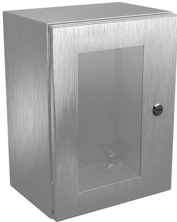
Wiegmann Ultimate series enclosure, NEMA 4/4X/12/13, 16 x 12 x 8in (HxWxD), wall mount, 304 stainless steel, No. 3 intermediate polished finish, single-door, 1/4-turn semi-flush oil-tight latch, polycarbonate window.
