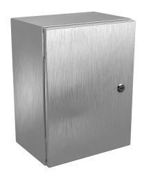
Wiegmann Ultimate series enclosure, NEMA 4/4X/12/13, 16 x 12 x 8in (HxWxD), wall mount, 304 stainless steel, No. 3 intermediate polished finish, single-door, 1/4-turn semi-flush oil-tight latch.
