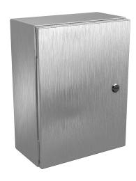
Wiegmann Ultimate series enclosure, NEMA 4/4X/12/13, 16 x 12 x 6in (HxWxD), wall mount, 304 stainless steel, No. 3 intermediate polished finish, single-door, 1/4-turn semi-flush oil-tight latch.
