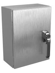
Wiegmann Ultimate series enclosure, NEMA 4X/12/13, 16 x 12 x 6in (HxWxD), wall mount, 316L stainless steel, No. 3 intermediate polished finish, single-door, 1-point 316L padlocking handle.
