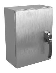
Wiegmann Ultimate series enclosure, NEMA 4X/12/13, 16 x 12 x 6in (HxWxD), wall mount, 304 stainless steel, No. 3 intermediate polished finish, single-door, 1-point 316L padlocking handle.
