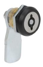
Wiegmann enclosure latch, double-bit key, 1/4-turn semi-flush, 1-point, vibration-proof, plated steel, black matte trim finish. For use with N412 Ultimate series enclosures. Requires N41214TVPK key.
