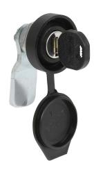
Wiegmann enclosure latch, keylocking, 1/4-turn semi-flush, 1-point, plated steel, black matte finish. For use with N412 Ultimate series enclosures. (2) keys and dust cover included.
