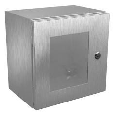
Wiegmann Ultimate series enclosure, NEMA 4/4X/12/13, 12 x 12 x 8in (HxWxD), wall mount, 304 stainless steel, No. 3 intermediate polished finish, single-door, 1/4-turn semi-flush oil-tight latch, polycarbonate window.
