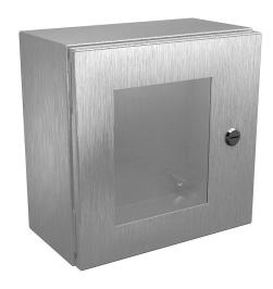
Wiegmann Ultimate series enclosure, NEMA 4/4X/12/13,  $12 \times 12 \times 6$  in (HxWxD), wall mount, 304 stainless steel, No. 3 intermediate polished finish, single-door, 1/4-turn semi-flush oil-tight latch, polycarbonate window.
